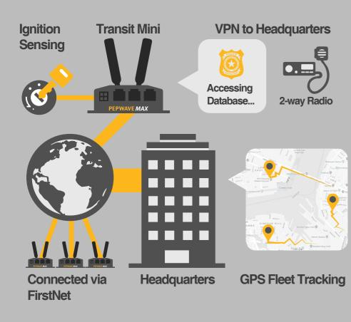
Using the MAX Transit Mini, officers on the field can connect to headquarters using FirstNet. Using the redundant SIM slot, the device can failover to commercial LTE as needed. By building a PepVPN to headquarters, 2-way radios such as TETRA, NXDN, and DMR can be used between multiple remote sites, enabling the entire force to seamlessly communicate as if they were connected to the same repeater. Finally, the Transit Mini can broadcast a mobile hotspot, connecting cameras and other equipment.
